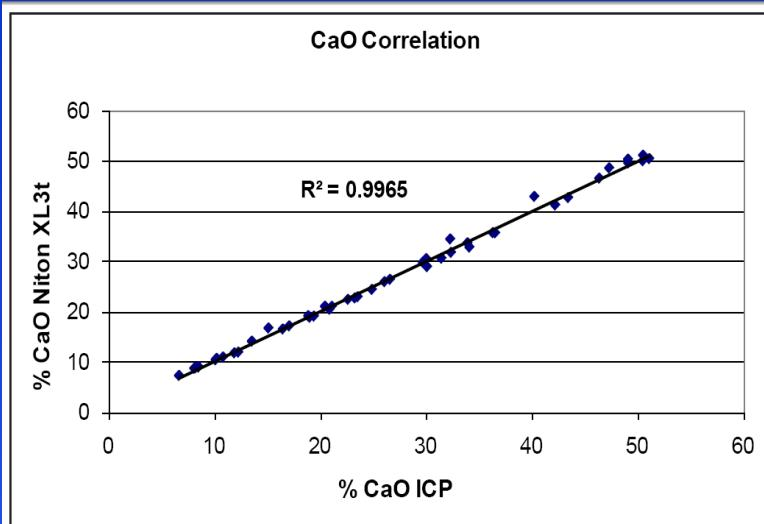
Figure 2. Correlation between CaO values measured by Niton XL3t Series analyzer and ICP-MS
