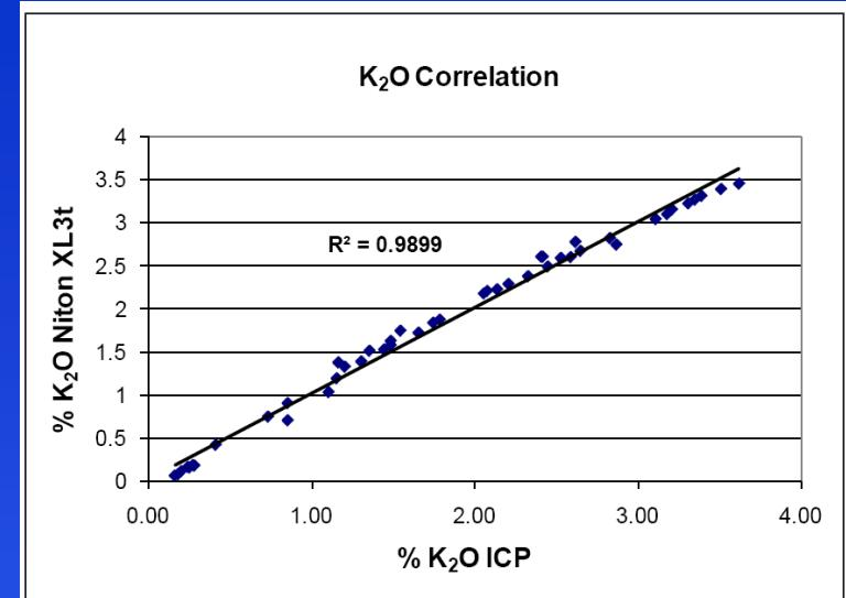
Figure 3. Correlation between K<sub>2</sub>O values measured by Niton XL3t Series analyzer and ICP-MS
