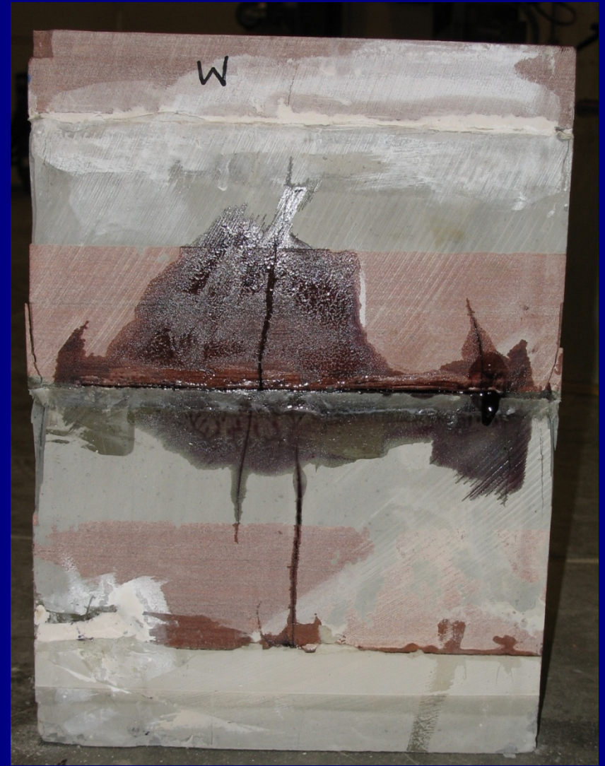
After hydraulic fracturing – notice the complexity for this “simple” system
