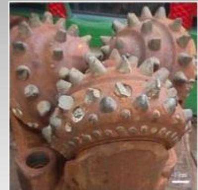
roller-cone with bits for oil drilling
